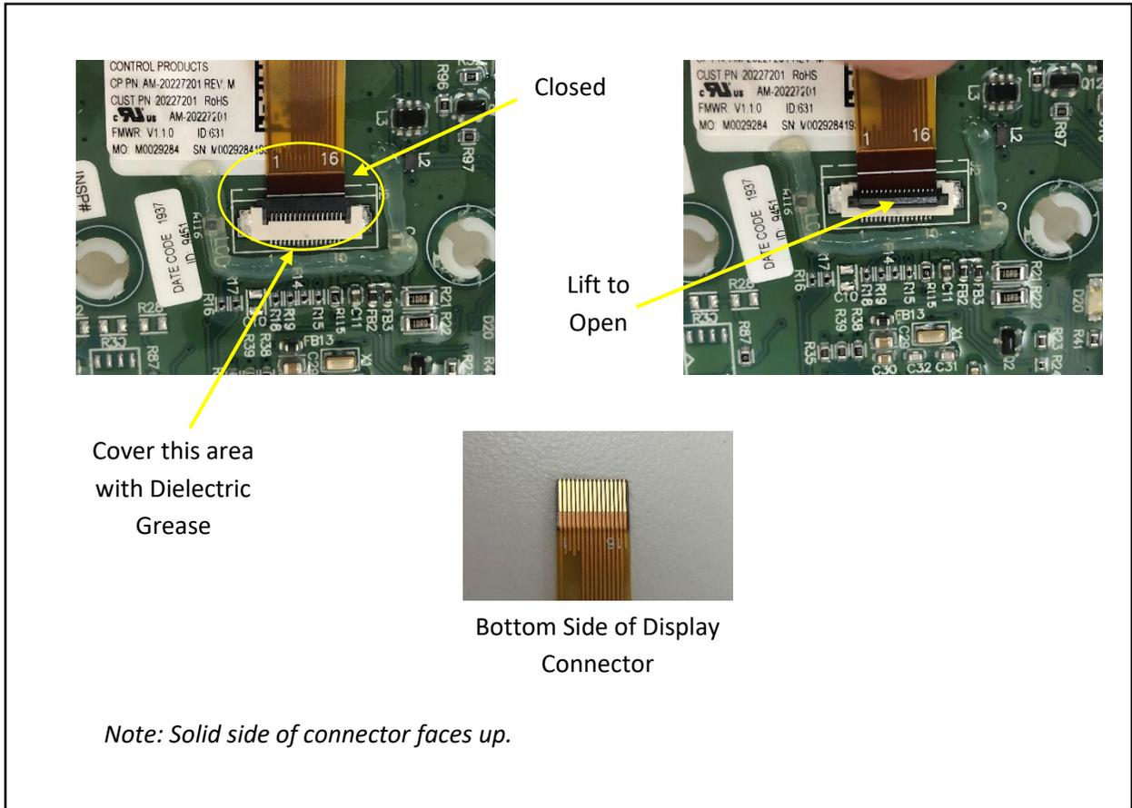
5. See **Figure 4**--Break protective strip (not USB port!) off new control board and place new Control Board in position to reinstall the Display Connector.
